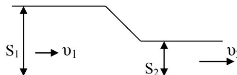
$$\frac{\rho v_1^2}{2} + P_1 = \frac{\rho v_2^2}{2} + P_2 \quad (1)$$
