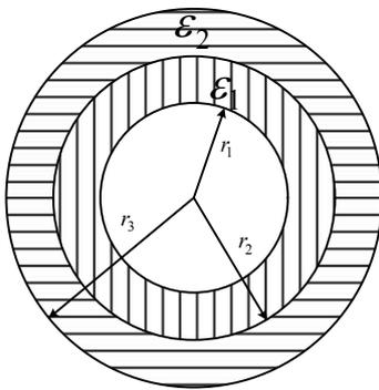
$$E_1 = \frac{U}{r_1 \ln \frac{r_2}{r_1}} \cdot \frac{C_2}{C_1 + C_2}; \quad E_2 = \frac{U}{r_2 \ln \frac{r_3}{r_2}} \cdot \frac{C_1}{C_1 + C_2}$$
