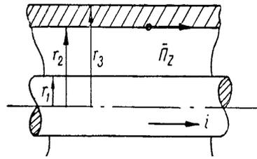
$$1. \Pi_z = \frac{U i}{2\pi r_1^2 \ln \frac{r_2}{r_1}}$$
