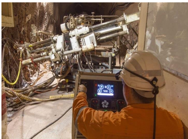
Figure 4. Semi-autonomous drilling by drill rig with Drill Control Interface
