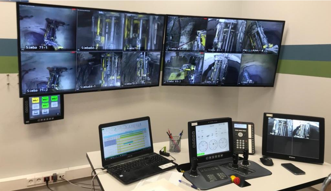
Figure 5. Semi-autonomous drilling to Kirovsky mine of Kirovsk branch of Apatit company.
