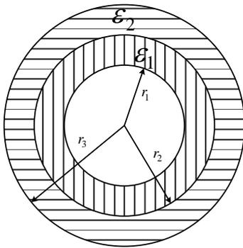
$$E_1 = \frac{U}{r_1 \ln \frac{r_2}{r_1}} \cdot \frac{C_2}{C_1 + C_2}; \quad E_2 = \frac{U}{r_2 \ln \frac{r_3}{r_2}} \cdot \frac{C_1}{C_1 + C_2}$$
