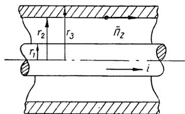
$$1. \Pi_z = \frac{ui}{2\pi r_1^2 \ln \frac{r_2}{r_1}}$$
